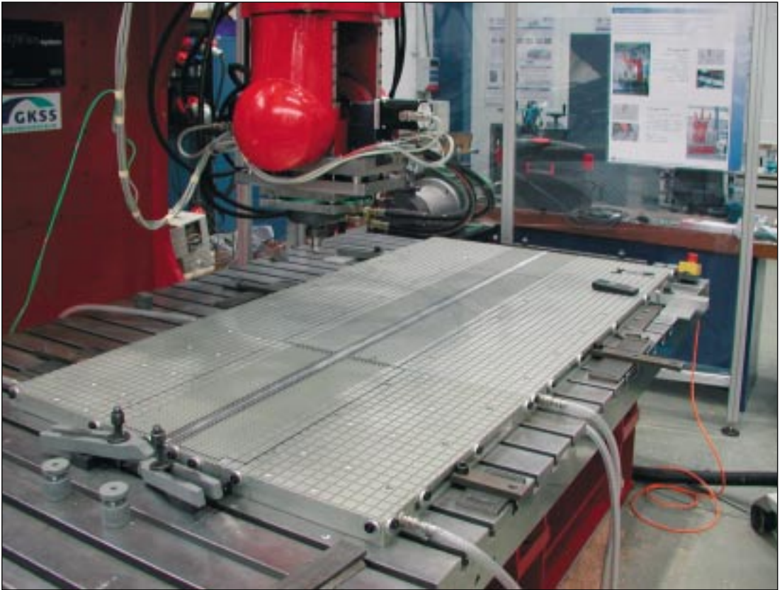
Combined METAPOR grid type chuck for friction stir welding application
