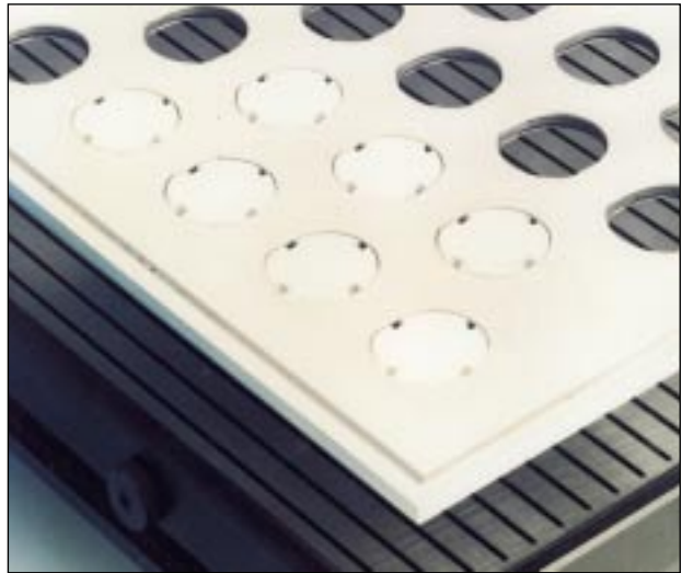
Slot vacuum chuck with special adapter plate
