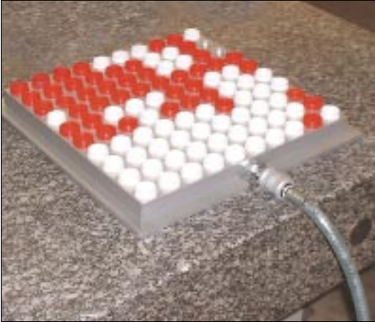
Vacuum chuck for bottle tops in quality control
