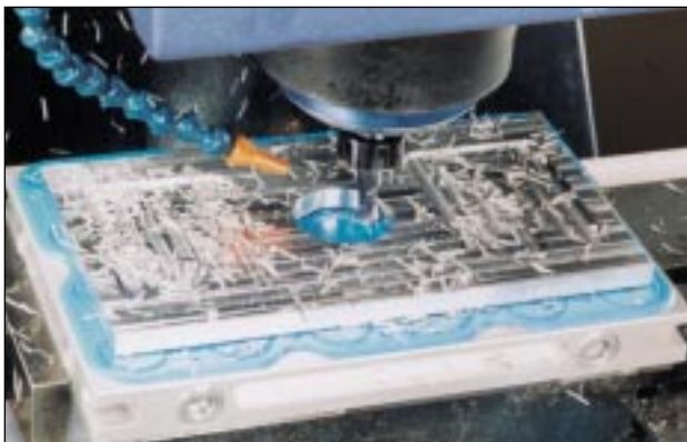
5 sided-milling an aperture on a VAC-MAT™ clamping system
